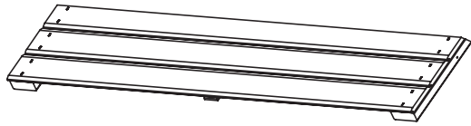
RP4 | ROOF PANEL ASSEMBLY-W2A03293 (x1) | 1 3/8"ax9 15/16"x40 15/16" (35x252x1040)
