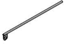
A4M00527 | GROUND STAKE REBAR (x2)
